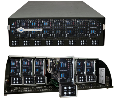
R4300 Chassis with 8 R3162D Blade PCs, 2 PCs per Blade for a total of 16 PCs in 3U chassis
